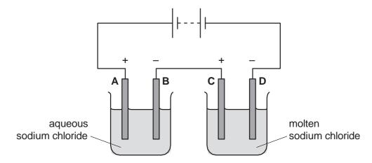
3 Concentrated aqueous sodium chloride is electrolysed using inert electrodes.
