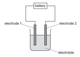
Which row shows the directions of movement of the electrons in the external circuit and of the positive ions in the electrolyte? **(extended only)**
